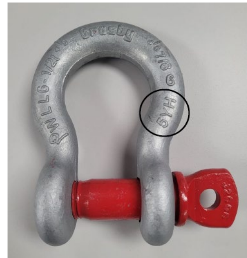
Figure 1. Recalled 7/8-in. shackle Photo: Crosby
