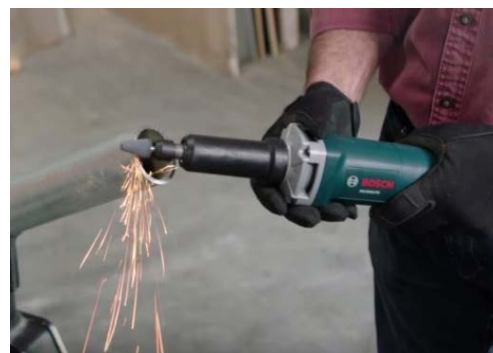
Die grinder (also called a pencil grinder).
