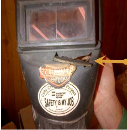
2014 -- Grinding wheel embedded in welding hood.
